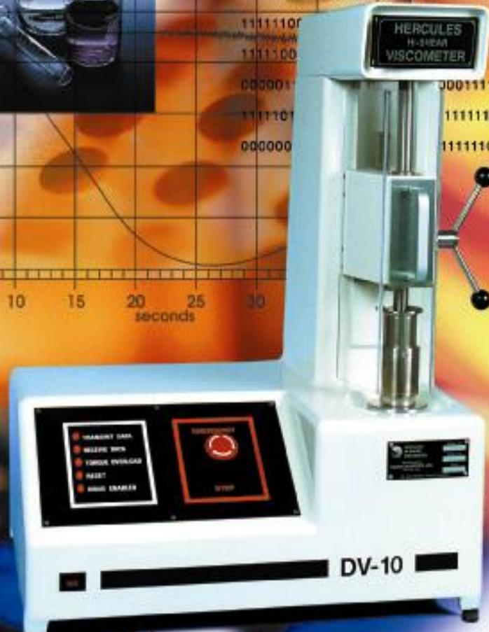
Generates shear rate ranges up to 185,000 sec<sup>-1</sup>
